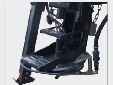
Wide steps integrated in the spreading disc arrangement mean safe and effortless access to the machine house.
