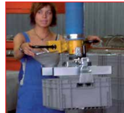
Mechanical gripper for crates with suspension clips
