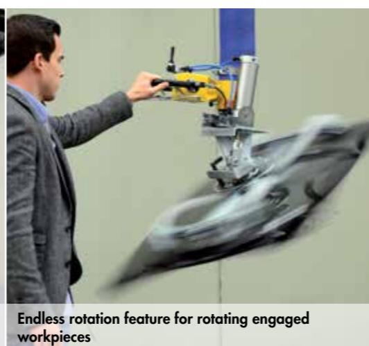
Endless rotation feature for rotating engaged workpieces
