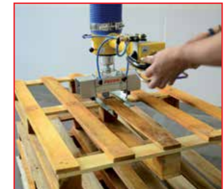
Pallet gripper with pneumatically adjustable undergrippers
