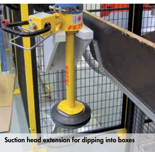
Suction head extension for dipping into boxes
