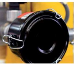
Large-dimensioned dust filter with exchangeable filter cartridge
