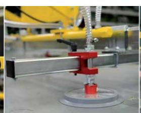
Suction pads with cross clamping piece to adjust on the cross beam
