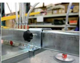
Mounting element with clamping screw to adjust the cross beam
