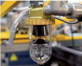
Water separator with manual drain for outdoors use or on water jet machines
