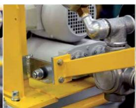
Swivel feature for angle adjustment of the manipulating handle
