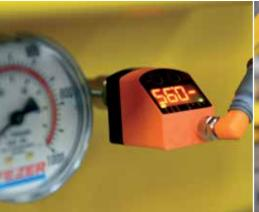
Vacuum-controlled motor switch to save energy and reduce the noise level
