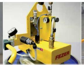
Air Pack: strictly running on compressed air via ejector and pneumatical warning unit
