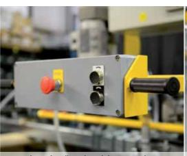
Manipulating handle with push-buttons and emergency-off on lifters with electrical movements
