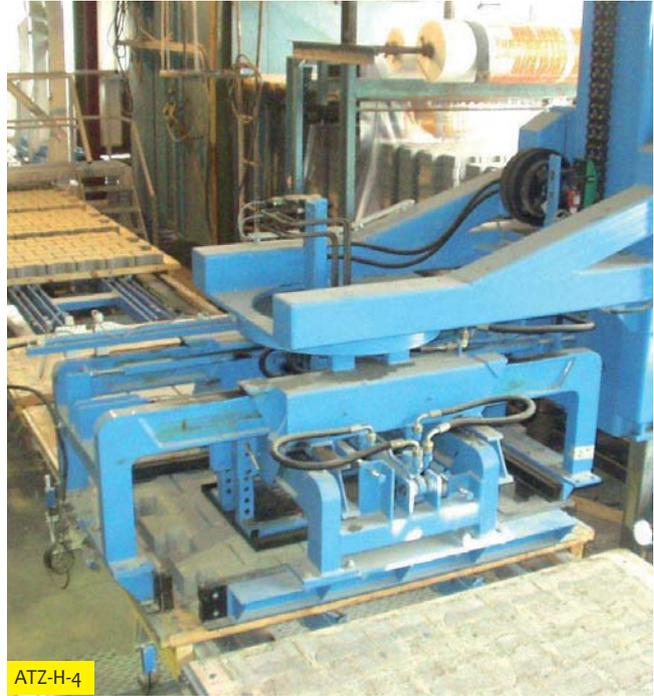
With the ATZ-H-4 hydraulic cubing clamp, very different combinations are possible.
