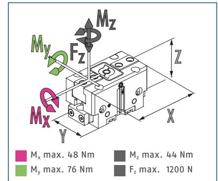
① The specified torques and forces are static values, apply for each base jaw, and may occur simultaneously.  $M_y$  may arise in addition to the moment generated by the gripping force itself.
