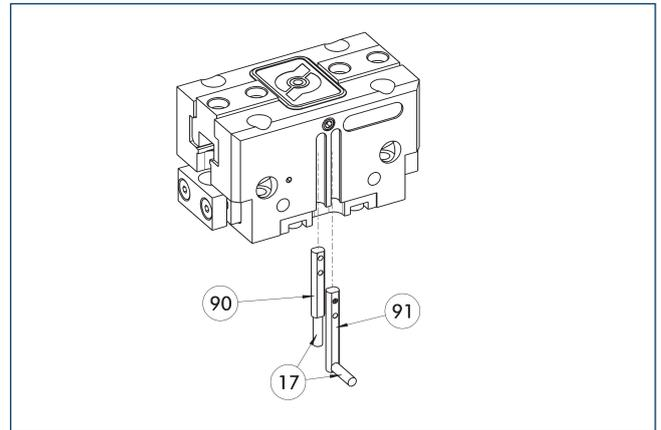
17 Cable outlet                      91 Sensor MMS 22...-SA
