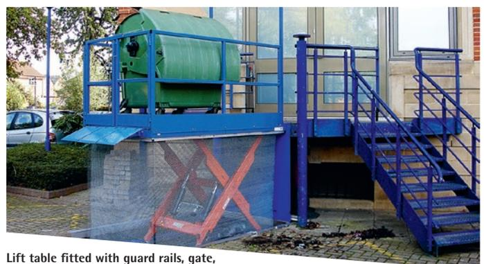
Lift table fitted with guard rails, gate, loadflap and protective wire mesh.
