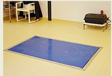
Lift table installed in a pit.
