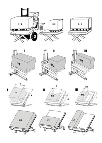
The stated lifting capacity of the lift table and pallet lifter required distributed load. TSL: Max. load = load centre 600 mm from column.
