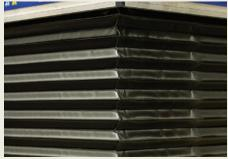
Protective bellows mounted on a lift table
