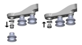
The thread size is the commonly used G1/8"; allowing for standard fittings, blinders and extenders to be fitted directly to the VG grippers.
