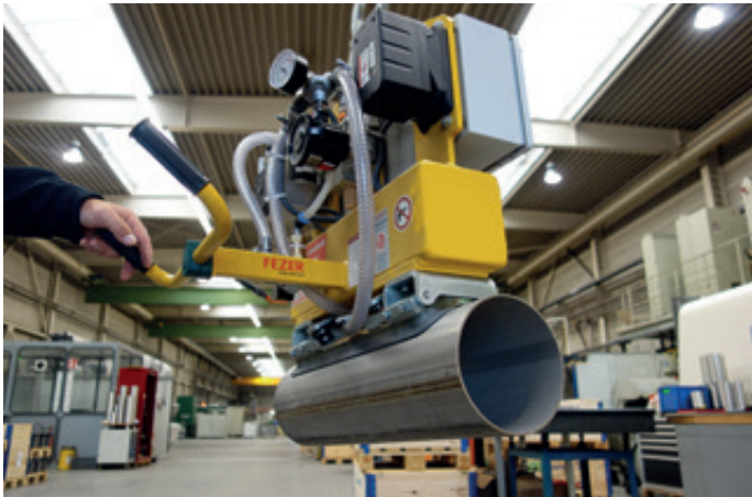
VacuBoyMini VBM-ACCU-50KG With articulated special grippers for transporting pipes with different diameters
