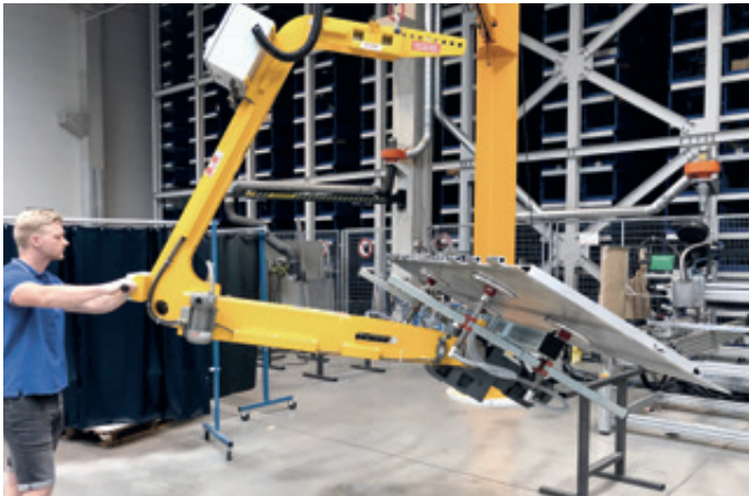
VacuBoy VB-180E-250KG Reversing on steel plates standing on edge
