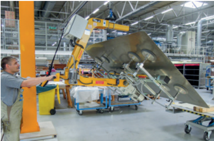
VacuBoy VB-180E-500KG For large steel plates up to 4,000x2,000 mm
