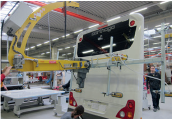
VacuBoy VB-180E-250KG For reversing and as an assembly aid for tail units for mobile homes
