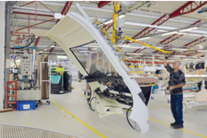
VacuBoy VB-90E-125KG For tilting mobile home front units
