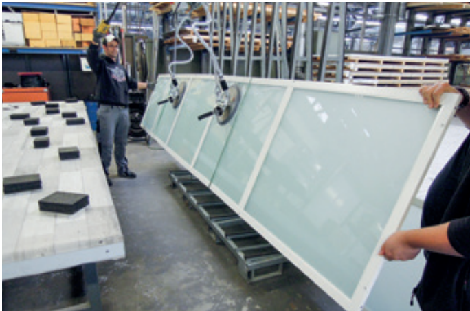
VacuBoyVario VBV-125KG Handling of window units up to 4,000 mm in length
