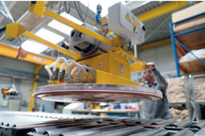
VacuCoil VC-500KG With plexiglass suction plate for simple centric placement on the split band rings
