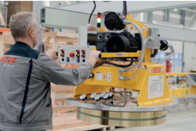
VacuCoil VC-500KG With a total of 5 suction chambers for accommodating coils with a diameter of 400-1,400 mm
