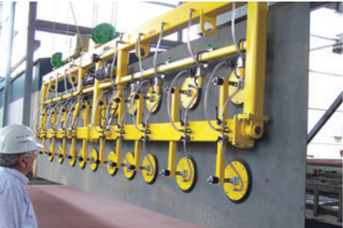
VacuGiant VG-90E-7500KG For large steel plates up to 4,000x2,000 mm
