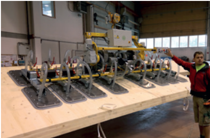
VacuGiant VG-90E-3500 For tilting wooden boards up to 250 mm thick
