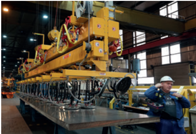
VacuGiant VG-12000KG-TEL Electrically telescopic vacuum traverse for loading a horizontal bar
