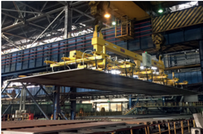
VacuGiant VG-25000KG For moving large-format sheets up to 20,000 x 3,500 x 50 mm
