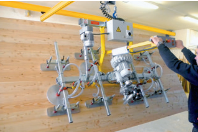
VacuPoro-90E-250KG For moving upright chipboard and OSB boards
