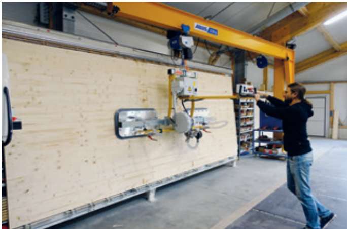
VacuPoro-90E-250KG For feeding a standing panel dividing saw
